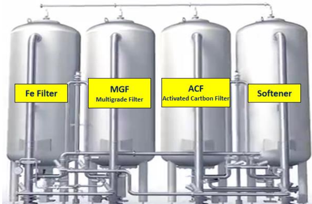
Figure: Water Treatment (Industrial Type)
