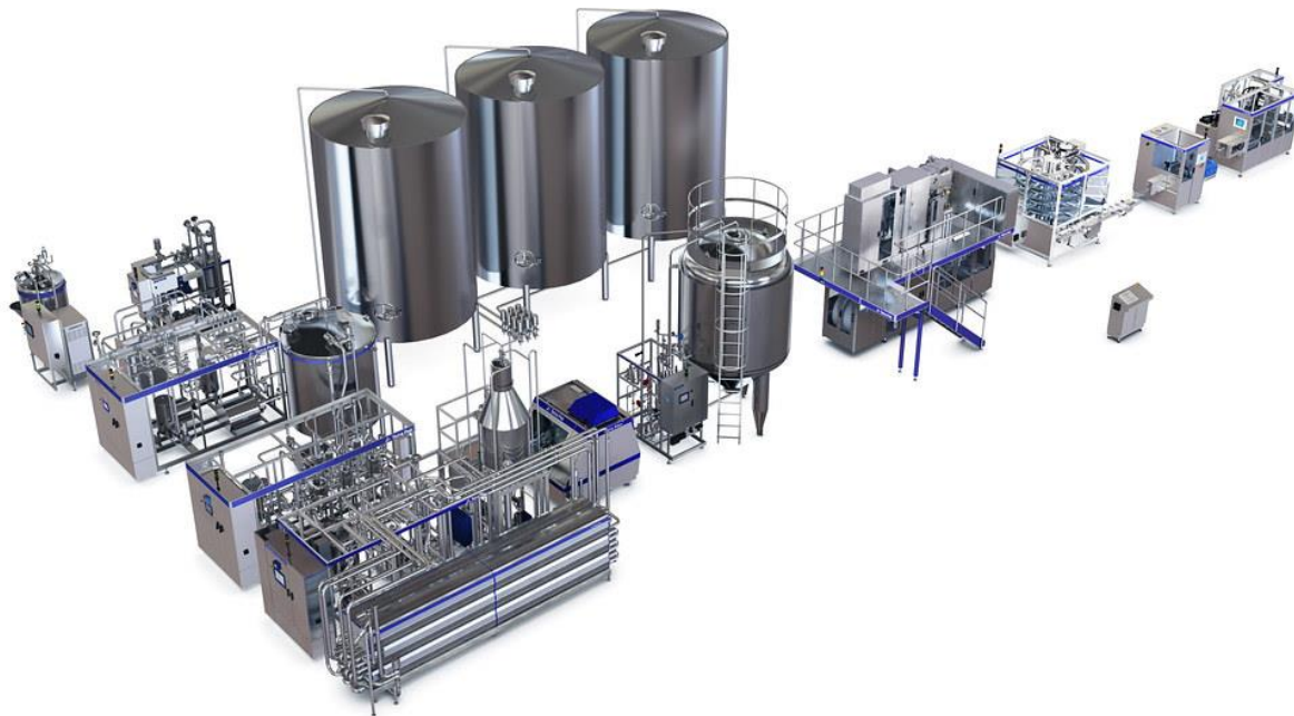
Figure: A processing unit including UHT system
