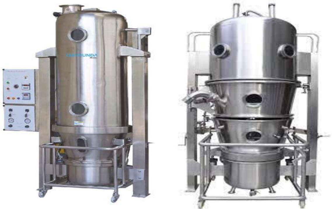
Figure: Fluid Bed Dryer
