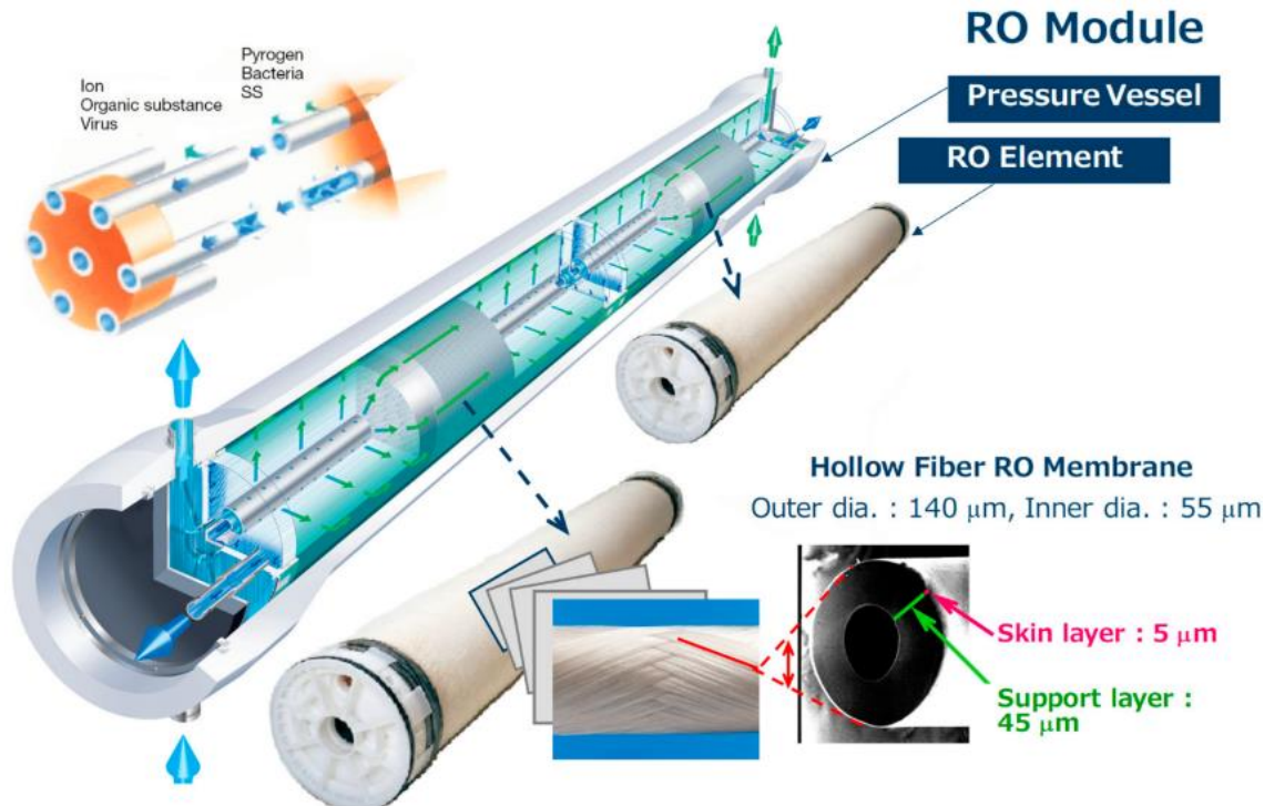
Figure: RO Membrane Piping
