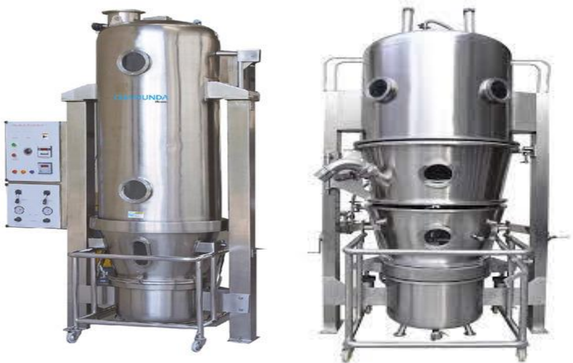
Figure: Fluid Bed Dryer
